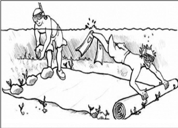
**Figure 22. A Benthic Barrier.** Photo courtesy of Cornell Cooperative Extension
