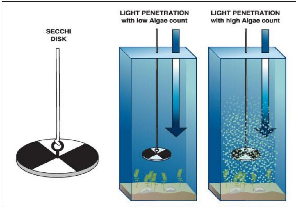
**Figure 7. A Secchi disk and the relationship between Secchi transparency and algae in the water column.**
