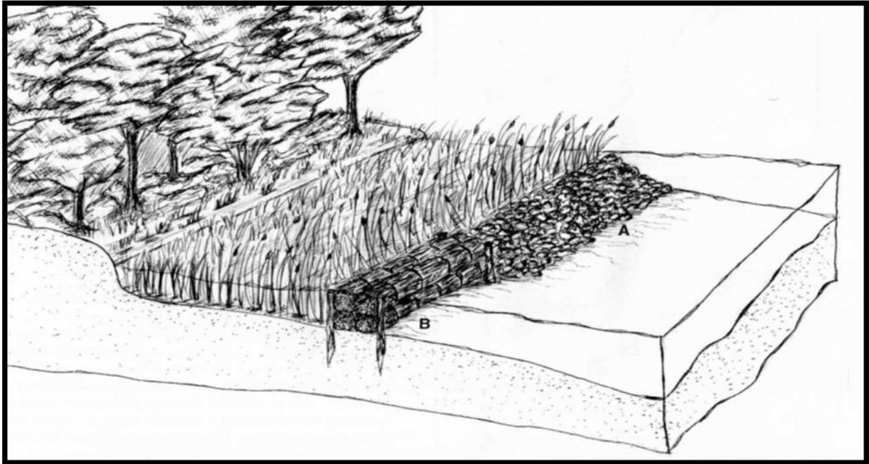
**Figure 38. Example of bioengineered shoreline restoration techniques. A) Rock rip-rap in combination with plantings. B) Willow bundles or coco coir logs in combination with plantings.**
