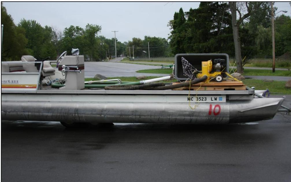
Figure 21. A DASH boat for hand-removal of milfoil or other nuisance vegetation. ©RLS
